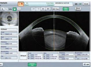
While capturing anterior cornea to posterior lens, it is possible to measure corneal curvature, thickness and tilt of the anterior / posterior lens.
